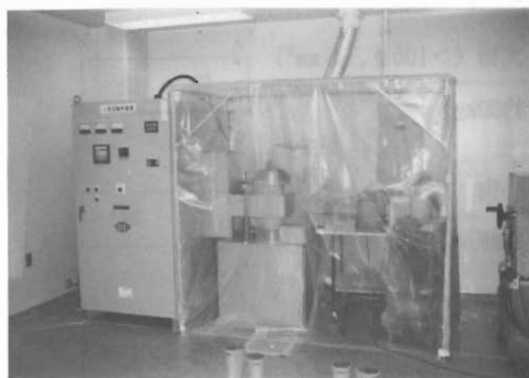
Photo 4 Hot test apparatus of induction heat melting.
